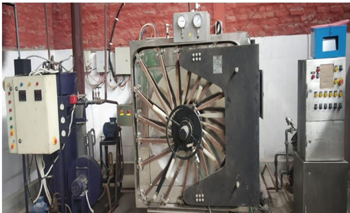
FIGURE 2.8 – HORIZONTAL CYLINDRICAL AUTOCLAVE & STERILIZATION PROCESS
